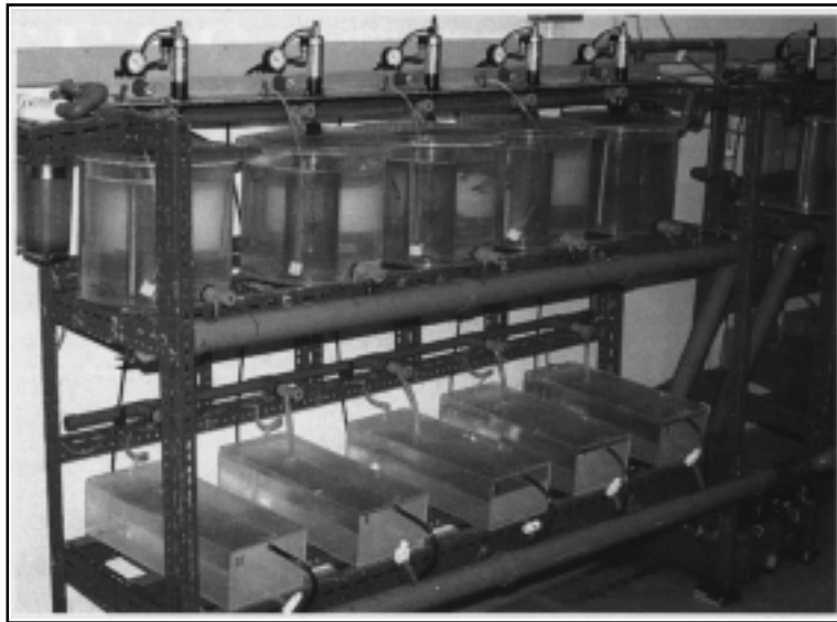
Figure 3. Sea Test apparatus set up showing agitation and recovery tanks
